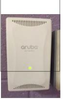
Pictured left are the newer Wireless Access Points that have been placed in some of the rooms on both campuses. If the light is off or not green, please contact the Help Desk. Stickers on the access points shown below will also have arrows that point to the (3) Ethernet jacks located on the bottom of the AP. These ports function as Regular wired room jacks.
